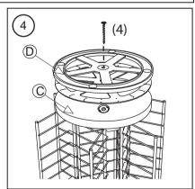
(4) Do not tighten screw too tightly. If base does not rotate easily, loosen screw.
